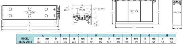
All dimensions in inches and (millimeters). All dimensions are for reference only. Contact a C&D Representative for complete dimensional information
